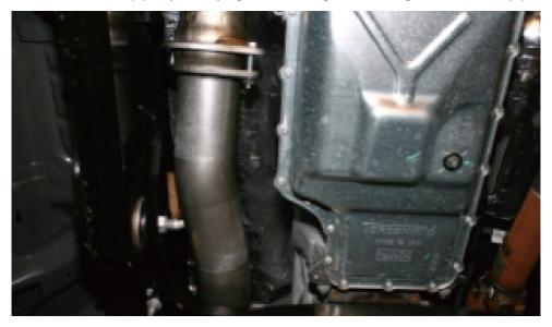
4. Next, install 61114NB pipe, placing hanger onto the OEM rubber mount and bolting the flanges together at the rear end.
