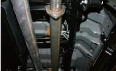
5. Next, install 61114NB pipe, placing hanger onto the OEM rubber mount and bolting the flanges together at the rear end.
