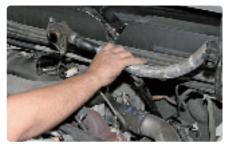
**Step 8:** Once both bolts are removed, the PCV hose assembly can be lifted out of the engine bay.
