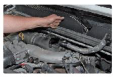
**Step 5:** The other end of the PCV hose is bolted to the turbo intake near the resonator delete plate as seen here.
