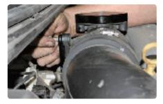
**Step 9:** Then install the included block off plate to replace the PCV hose assembly and reuse the factory mounting bolts to secure the plate. Be sure to position the wire harness bracket under the lower bolt once again so that it is secure in the engine bay as shown.
