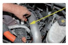
**Step 4:** After removed the clamp, pulled the end of the PCV hose off the fitting as shown.
