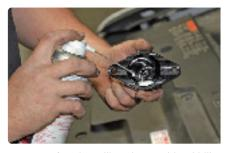
**Step 1:** Before installing the machined billet aluminum delete plate, lubricant on the inside and runs it around the inner edge with his finger to prevent it from snagging on the 0-ring as it's installed.
