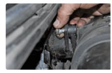
**Step 6:** After loosening the top bolt, it can be threaded out by hand.
