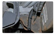
**Step 14:** Lift the truck on the hoist and go under it to route the hose to the outside of the frame, and then secure it with the zip-ties provided in the kit. Installing a vented catch can with a drain and breather filter would be a good addition to the PCV reroute especially for anyone interested in drag racing their truck.
