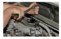
**Step 2:** Tightens the mounting bolts to the plate. Be sure not to over-tighten them as they are running into a plastic intake tube and the 0-ring handles the seal, not the torque on the bolts.
