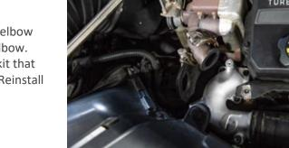
STEP 20: Install the coolant bypass hose to the coolant bypass elbow.
