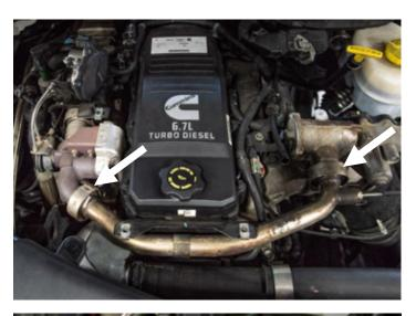
STEP 13: Remove the 8 mm bolt that retains the cross over tube at the front of the engine.
