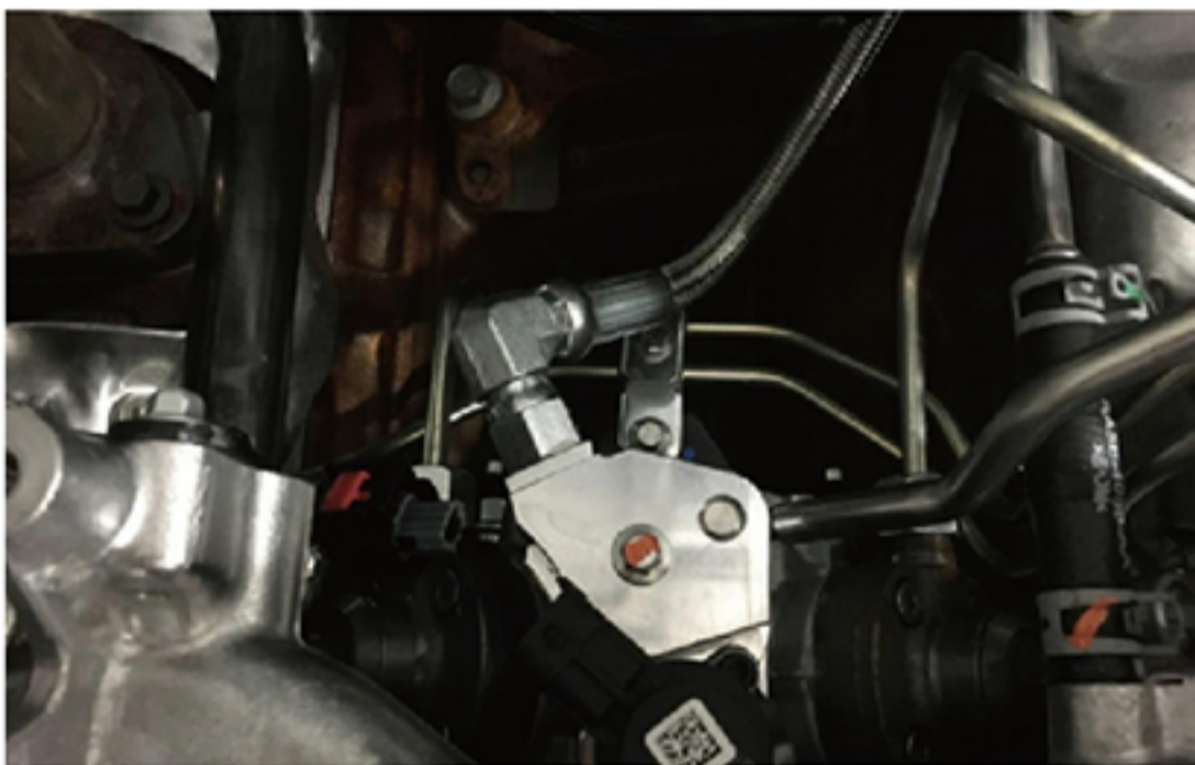
Note this braided line must not touch any component as it is fit into the valley and run out.
