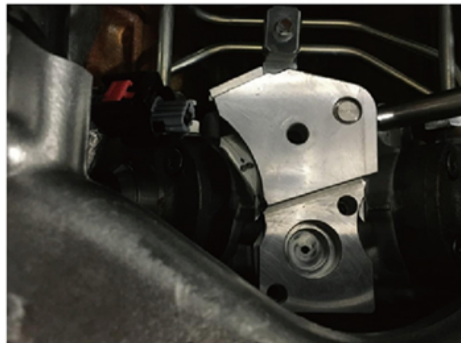
Install metering unit (FCA) and tighten all fasteners
