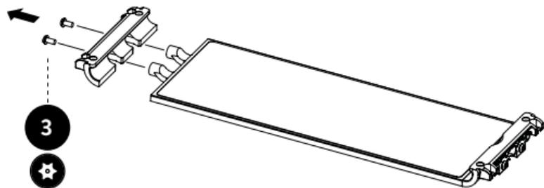
3. Use the Security Tool to remove the 2 screws holding the end cap in.
