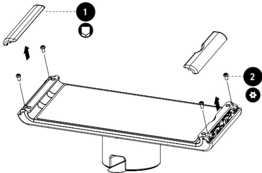
1. Use the Pick Tool to lift off the metal end caps from the Lock Belt.
