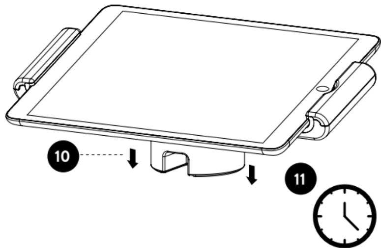
**10.** Press down firmly on the base to adhere the stand in place.
