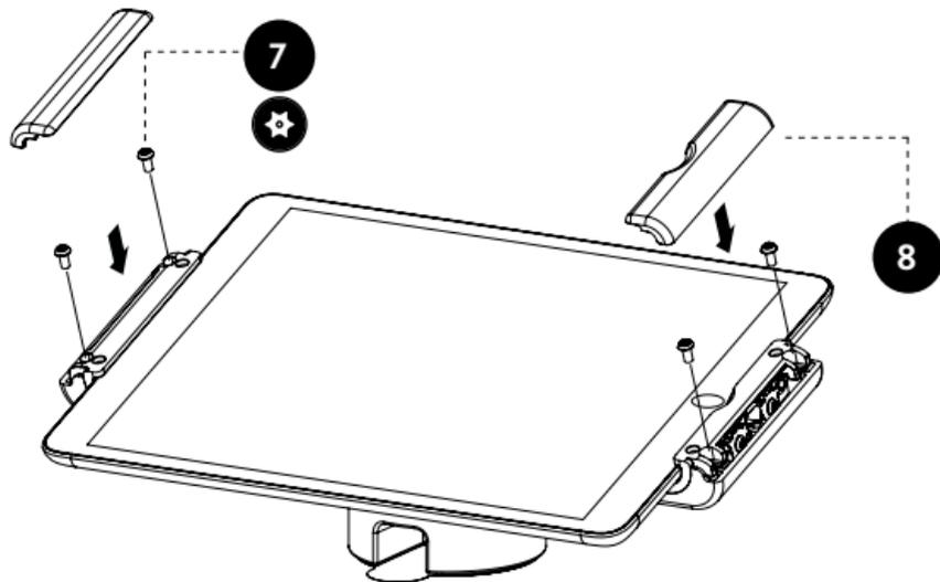
7. Use the Security Tool to attach the iPad to the frame.
