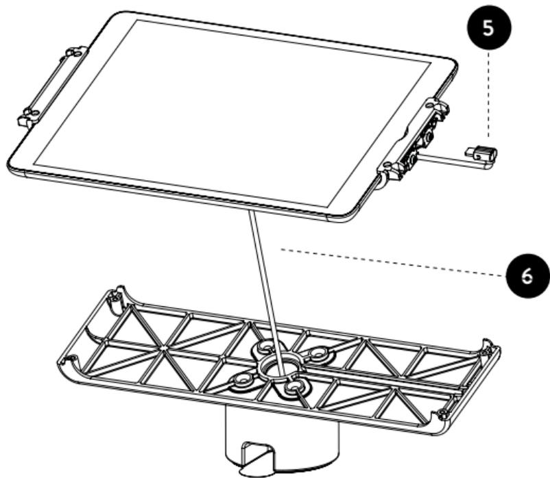
5. Connect the Lightning cable to the iPad. There are clips underneath to hold it in place.
