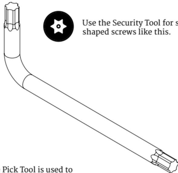
Use the Security Tool for star shaped screws like this.
