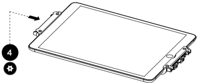
4. Position the iPad into the frame and tighten with the security screws.
