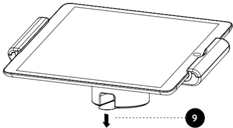
9. Peel the backing off the adhesive base.
