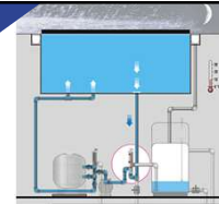
Backwash from bottom drain
