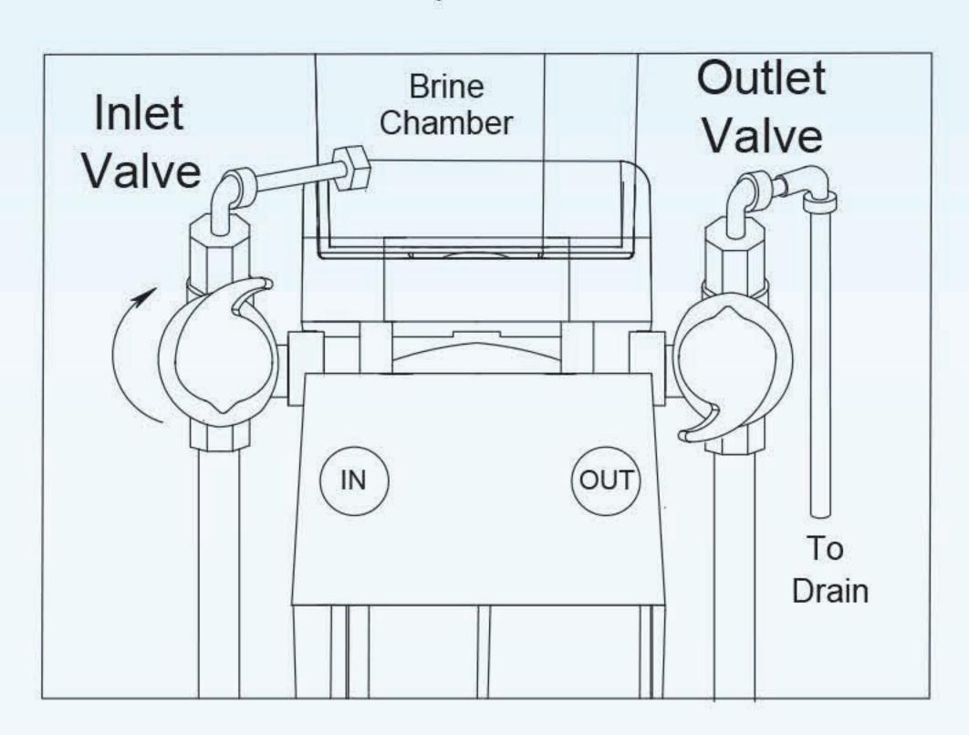
After 5 minutes, rotate the outlet valve anti-clockwise and bring it back to its original position (facing upwards). During this time, the regenerated water would be drained out through outlet pipe (1/4").
