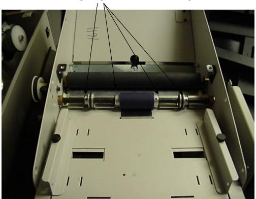
Loosen, but do not remove, the set screws on the feed wheel and guide rollers.
