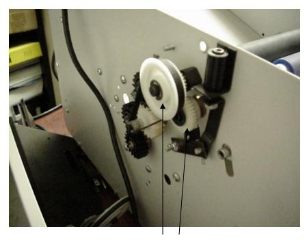
Remove the two top gears
