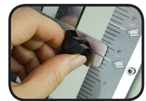
Align the fold stop notch with the icon that matches the fold type and paper size.
