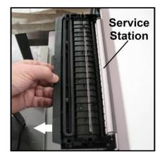
Disconnect the Ribbon Cable. Slide the Latch open on the Service Station Circuit Board to release the Ribbon Cable.
