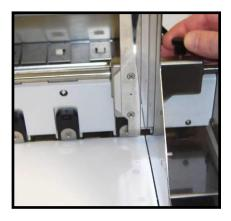
7. Adjust the position of the Rear Media Support Guide, so that it is centered under the width of your media. This guide slides side to side.
