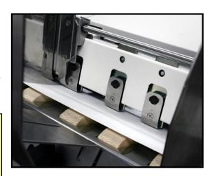
**6.** Loosen the locking knob and reposition the Adjustable Media Side Guide so that it is about 1/32-inch from the side of the media. Then tighten the locking knob to secure the side guide.
