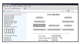
3. Click the button labeld "Replace Ink Tanks", located in the Toolbox User Interface screen. This disconnects Printer communication with the Ink Tanks and allows safe installation and replacement.
