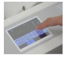
**TOUCH SCREEN** The LED touch screen sets up 36 standard folds automatically at the touch of a button. Up to 12 custom folds can be stored in memory.
