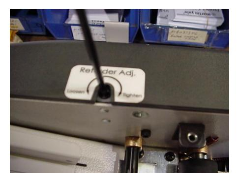
If the retarder pressure is too light turn the wrench toward TIGHTEN while moving the paper. When you feel the paper being pinched the adjustment is complete.
