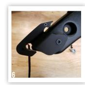
Plug in plate light connector and run harnesses back to factory location under seat and plug in
