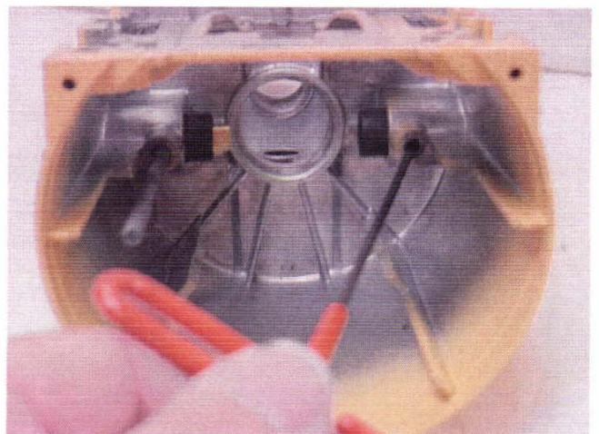
Fig. 33 Removing the brush holder set screws with an allen wrench.
