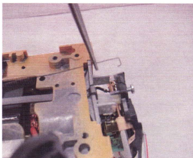
Fig. 50 The control plate spring being grasped with pliers and positioning the hook into the hole at the bottom.
