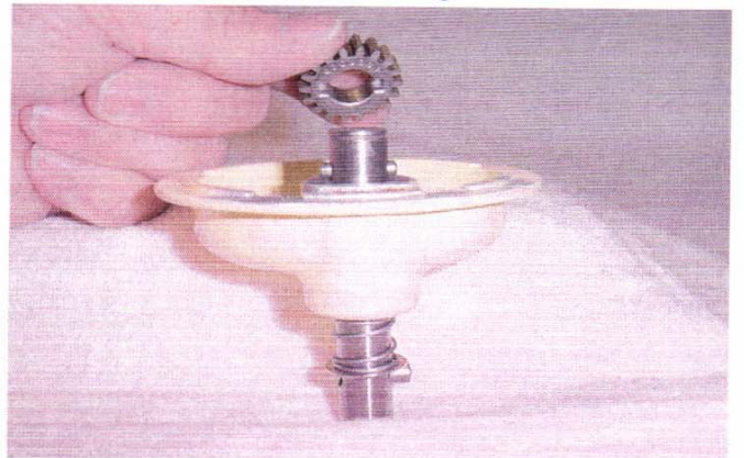
Fig. 65 Lift the pinion off and take out the pin and remove the washer; then pull out the shaft.
