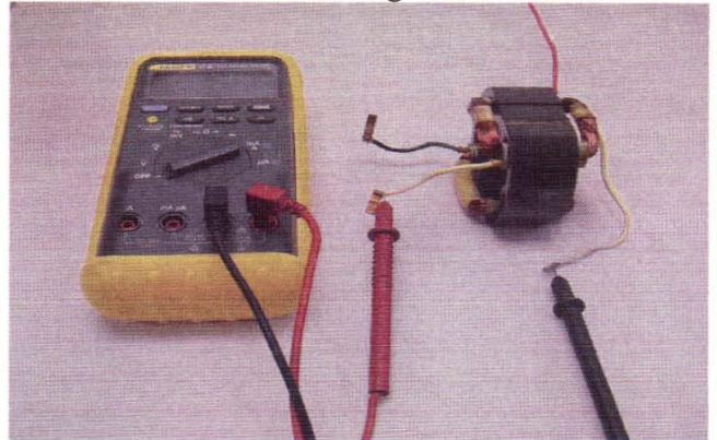
Fig. 35 Test the two stator coils with an ohmmeter set on low scale.
