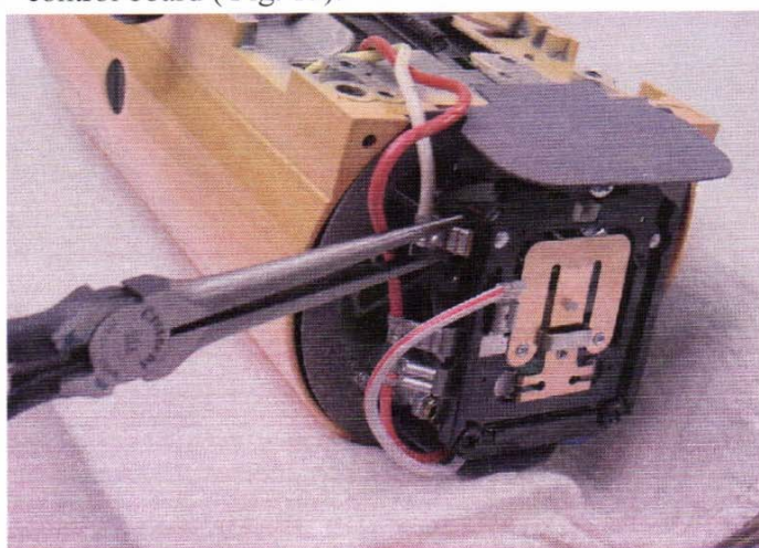
Fig. 15 The removal of the motor stator flag terminals from the control board.
