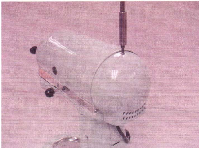
Fig. 1 The end cover is removed by removing the tapered head endcover screw.
