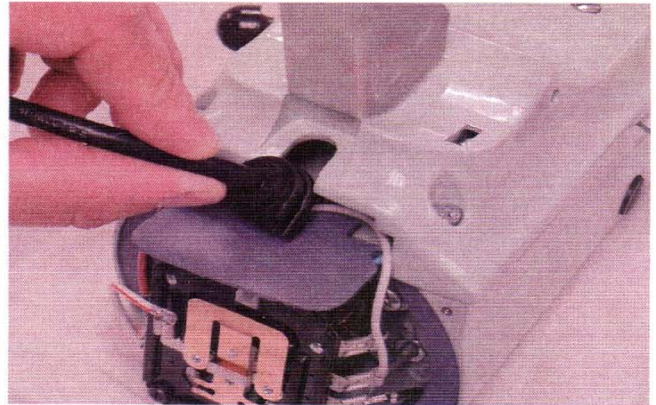
Fig. 8 Pull back on the molded strain relief to remove the power cord from the slot in the bottom cover.
