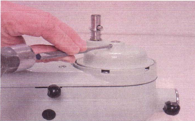
Fig. 6 Removal of the groove pin that holds the planetary to the vertical center shaft
