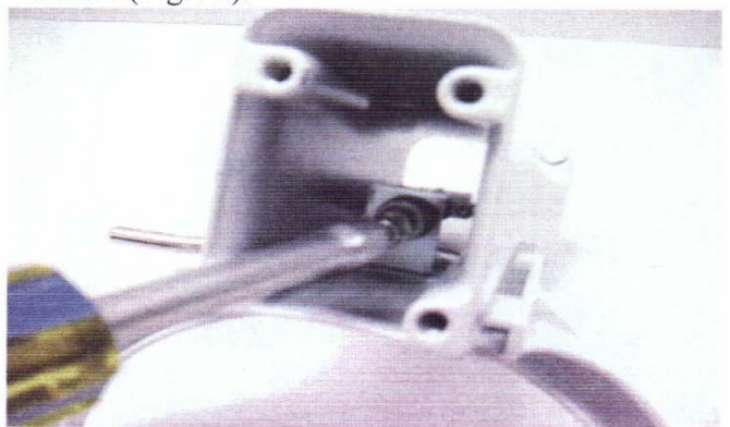
Fig. 92 Check the castle nut for proper tension on the bowl lift bracket.
