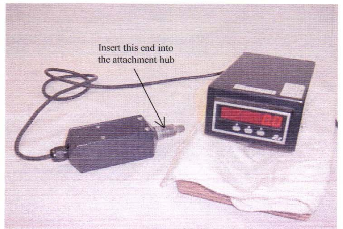
Fig. 80 Electronic speed measuring device, with numerical display for setting speeds on KitchenAid mixers.
