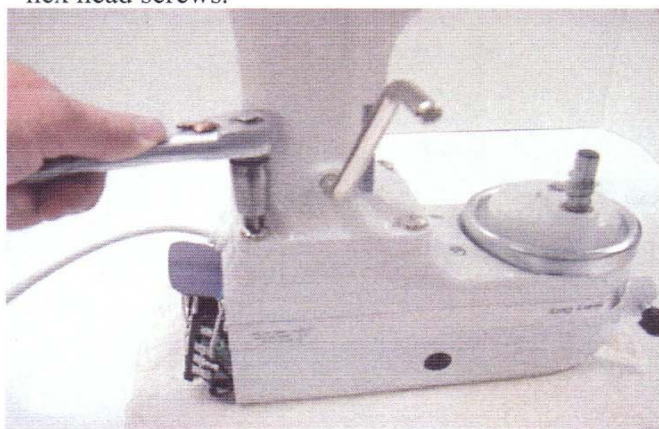
Fig. 84 Four round Phillips head screws must be removed to replace the bowl support assembly.
