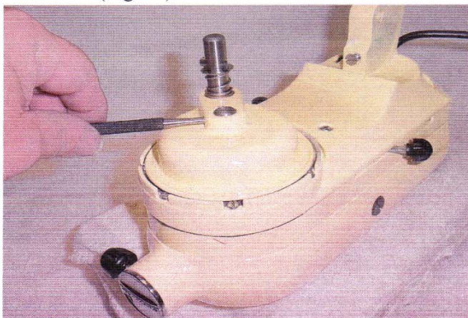
Fig. 67 A pointed punch can be used to align the holes of the shaft with the planetary.
