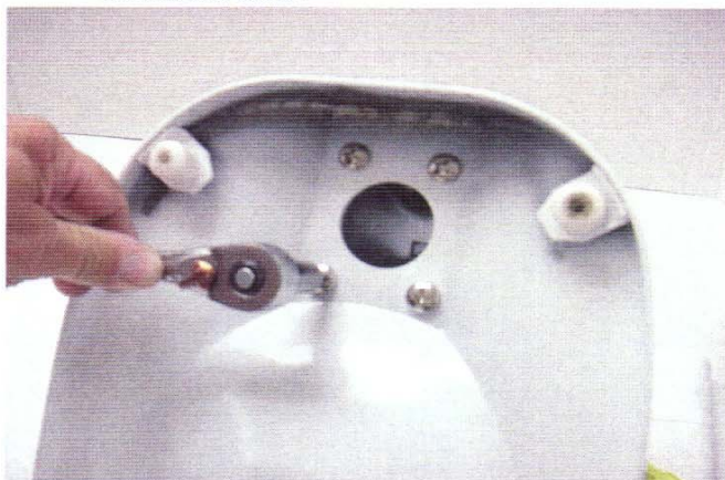
Fig. 86 Remove the four round head screws from the base to remove the bowl lift assembly.
