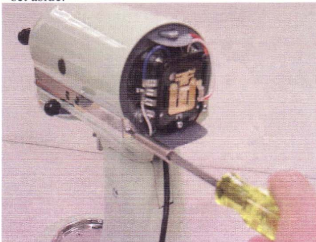
Fig. 2 The trimband can be removed after removing the trimband screws.
