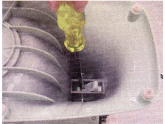
Fig. 3 Loosen the hinge pin setscrew to remove the pedestal from the bottomcover.
