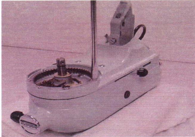
Fig. 10 Removal of the 5 special screws holding the internal gear in the bottom cover.
