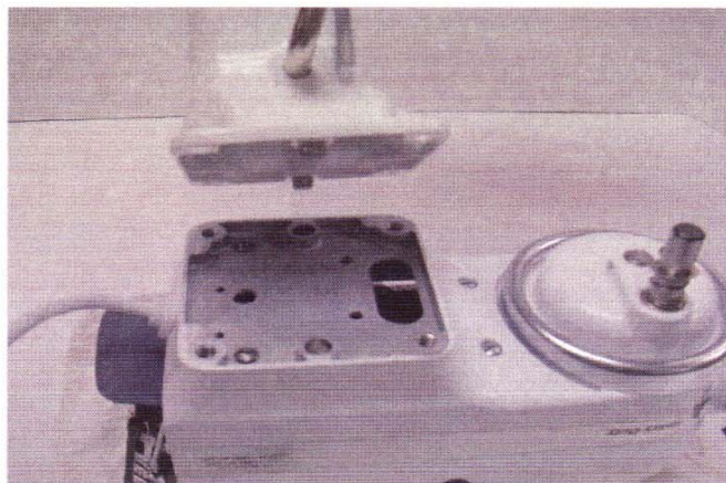
Fig. 85 Lift the column and bowl support assembly off of the bottom cover.
