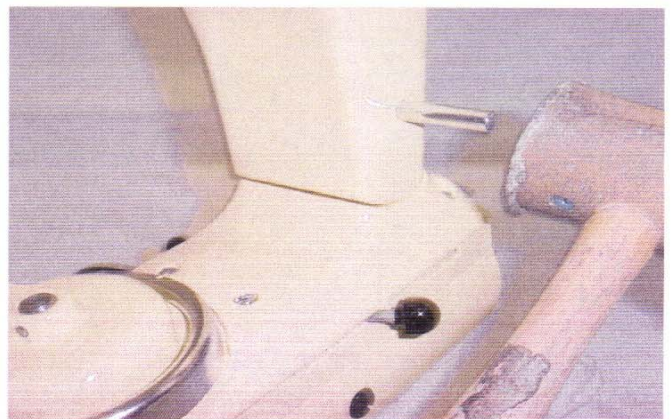
Fig. 73 Use a rubber or rawhide mallet to tap the hinge pin into the pedestal.
