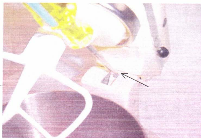
Fig. 83 The beater height adjustment screw used to set the 1/16" clearance between the bowl and beater.
