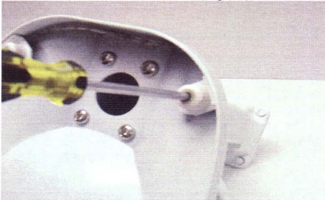
Fig. 93 Remove the four round head screws to remove the feet from older models.
