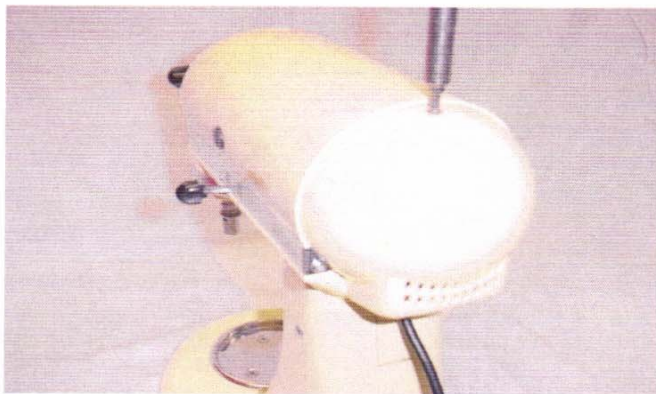
Fig. 82. The end cover is secured to the mixer with a tapered head screw.
