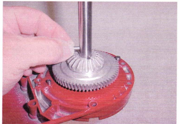
Fig. 53 Remove pin after pushing vertical center shaft up.
