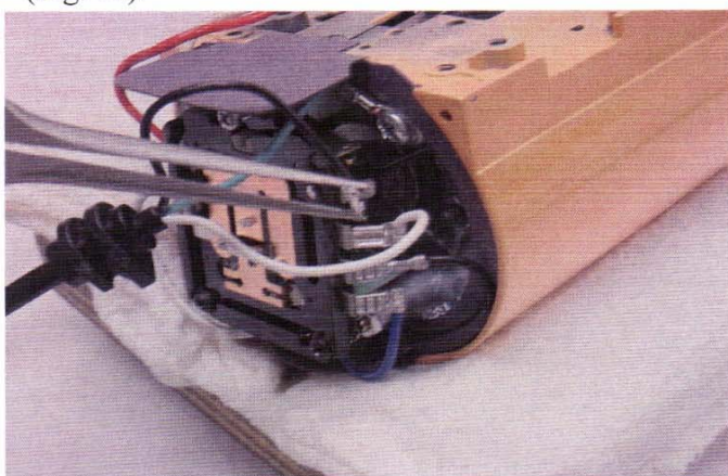
Fig. 14 Removal of the cord flag terminals and cord ground wire.
