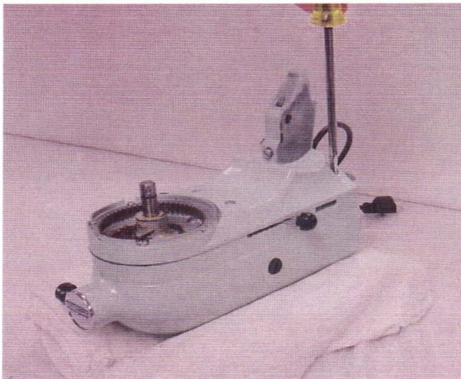
Fig. 11 The bottom cover is removed after removing the four #10-24 filister head screws.
