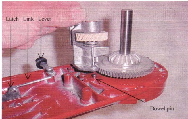
Fig. 58 The two dowels must fit into the base of the worm gear bracket.
