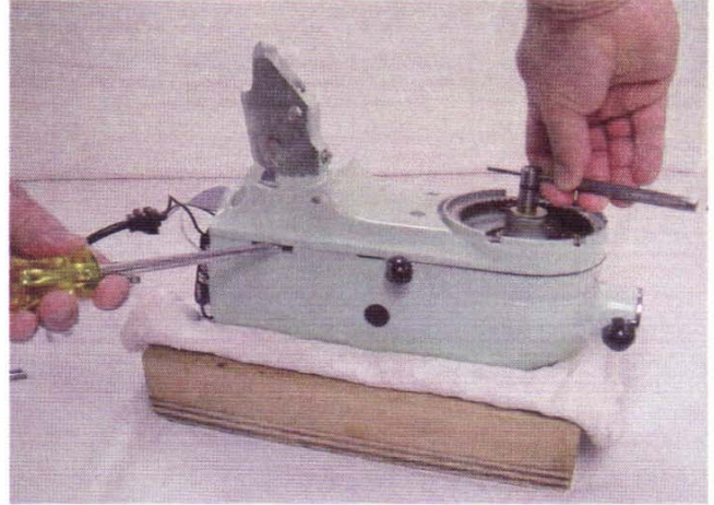
Fig. 12 While lifting up on the center shaft, use a screw driver to gently pry the bottom cover from the housing.
