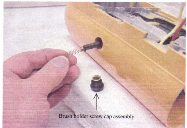
Fig. 42 Placing one of the brushes into the mixer brush holder.
