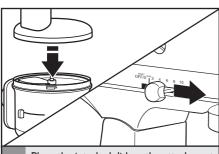
Place the interlock lid on the attachment assembly, making sure to click the lock into place. Turn on the Stand Mixer on to the appropriate speed. See the Speed selection guide for more information
