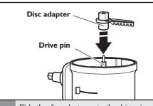
2 Slide the disc adapter onto the drive pin.
