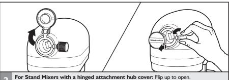
For Stand Mixers with a hinged attachment hub cover: Flip up to open.
