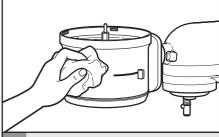
Wipe the attachment assembly with a warm, damp cloth. Avoid using abrasive cleaners or scouring pads as they may scratch the attachment assembly casing. Thoroughly dry with a soft cloth. To avoid damaging the Food Processor attachment, do not wash or immerse the attachment assembly in water or other liquids.
