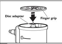
Hold the reversible shredding disc by the 2 finger grips with the desired shredding side facing UP. Install the disc on the disc adapter by fitting the adapter through the hole in the bottom of the disc until it is seated against the liner.
