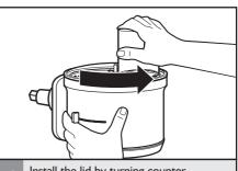
Install the lid by turning counter clockwise, being sure it locks into place.
