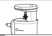
Insert the liner into the attachment assembly so that the feed tubes line up and the liner lies flat.
