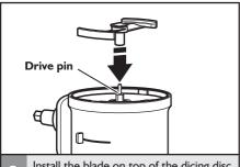
Install the blade on top of the dicing disc by sliding it onto the drive pin.
