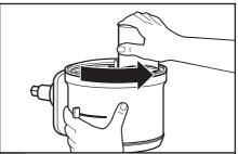
Install the lid by turning counter clockwise, being sure it locks into place.
