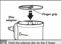
Hold the julienne disc by the 2 finger 3 grips, with the smaller side of the middle hole facing UP. Install the disc on the disc adapter by fitting the adapter through the hole in the bottom of the disc until it is seated against the liner.
