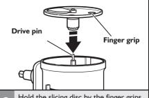
Hold the slicing disc by the finger grips 2 and lower it onto the drive pin. You may need to turn the disc/drive adapter until it drops down into place.
