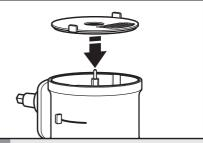
Hold the dicing disc by the middle hole and disc edge, chute lip-side facing DOWN. Place the disc on top of the liner so that the dicing grate aligns with the liner's feed tube.
