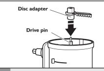
Slide the disc adapter onto the drive pin.
