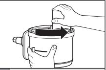
Install the lid by turning counter clockwise, being sure it locks into place.
