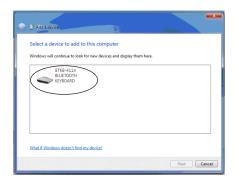
5. Using the Bluetooth keyboard to type the passkey provided by your system on the screen, press **Enter** on your keyboard and click **Next.**
