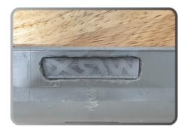
7.Take the LED Housing and adhere it to the back of the shifter trim with the wire facing the driver's side of he vehicle.
