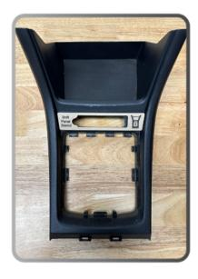
9.Place the control box on the inside of the shifter area out of the way using the supplied 3M adhesive and feed the power and ground wires through the driver's side footwell panel, runing them to the interior fuse box.
