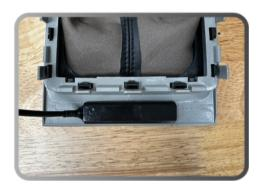
8.Apply the Shift Panel Stencil to the area beneath where the shifter trim rests and mark the area to be trimmed.
