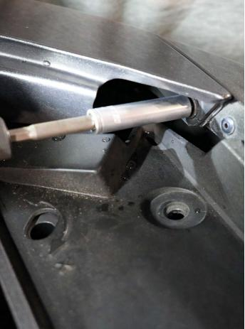
Extract the four push-in pins from both sides of the wheel fender.
