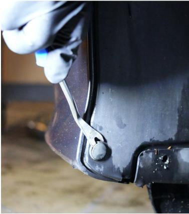
Subsequently, spread open the fender liner widely and use the wrench to disengage the two 10mm bolts securing the front bumper.
