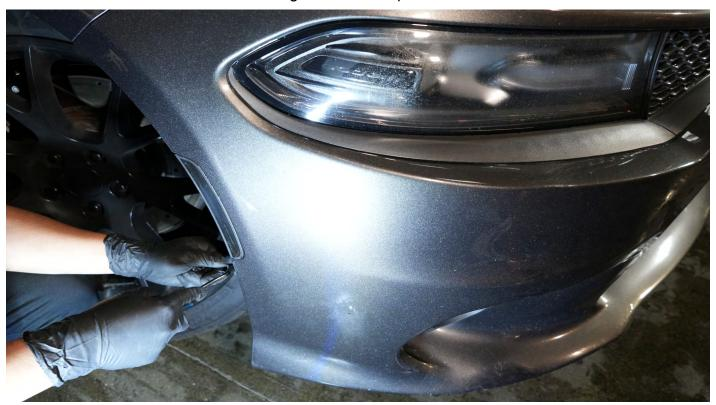
Take out the eight 7mm bolts located underneath the front bumper.
