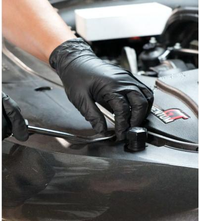
Remove the two 10mm bolts, located individually on either side of the upper bumper corner.
