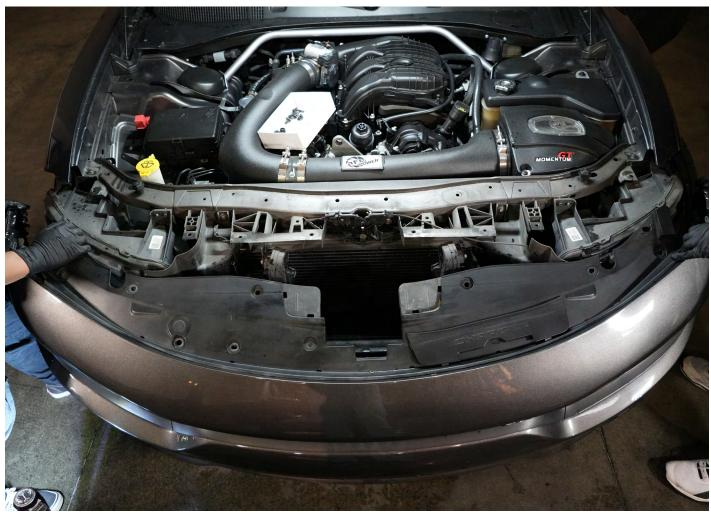
Disconnect the fog light connectors and side marker connectors, then proceed to remove the front bumper entirely. Set it aside for later reinstallation.
