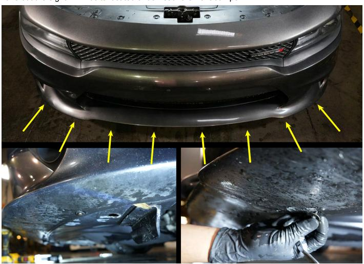
Gently detach the front bumper by pulling outward from each side, disengaging it from the mounting clips.
