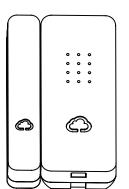
**Step 3**. Move the magnet in contact with the Reed KumoSensor and then away. A LED light should start flashing for about 2 minutes. Search and assocaite during that time.
