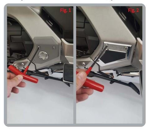
3. Determine correct orientation for the left and right sides of the motorcycle. Install covers using original screws, torque to 5.2 N-m, 3.8 ft-lbs. Do not overtighten. (Fig. 2)
