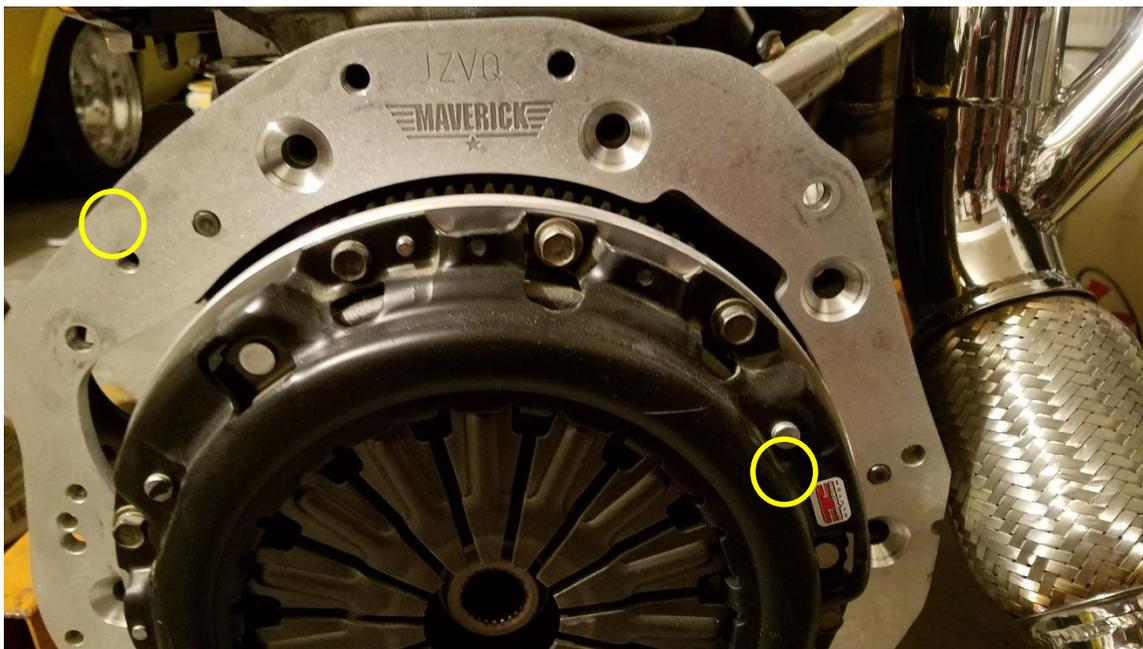
Use the provided countersunk bolts to attach to the engine.
