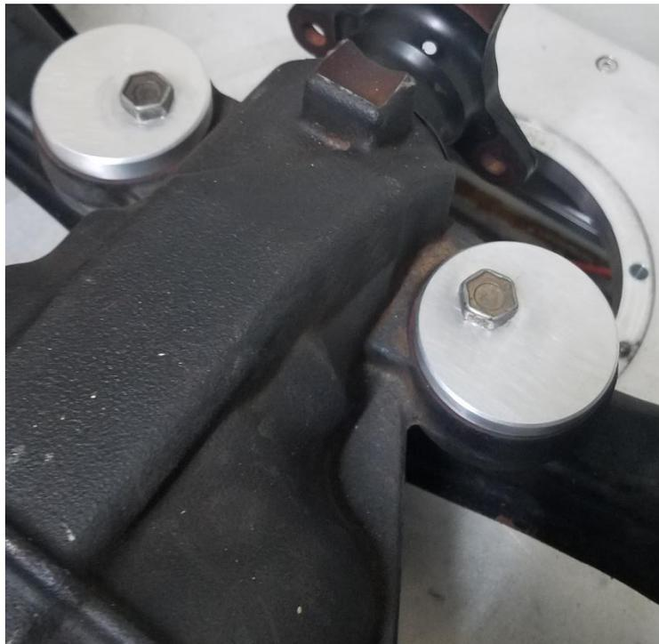
**Step 9:** Driveshaft fitment: Take your driveshaft and place it against the diff flange. The 350z uses a larger input pinion flange and it must be re-drilled to match the S-chassis driveshaft. Re-drill the 4 bolt holes to match your driveshaft.
