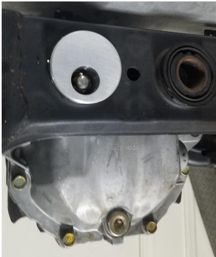
**Step 7:** Now comes the hardest part. Hoist the diff into the subframe and align the rear stud with the rear bushing. Use a nut or a bolt to help “pull” the diff back while constantly supporting it with the jack. Raise the diff until its flanges are flush with the subframe.
