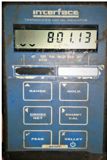
Photo 4 – Load Cell Readout
