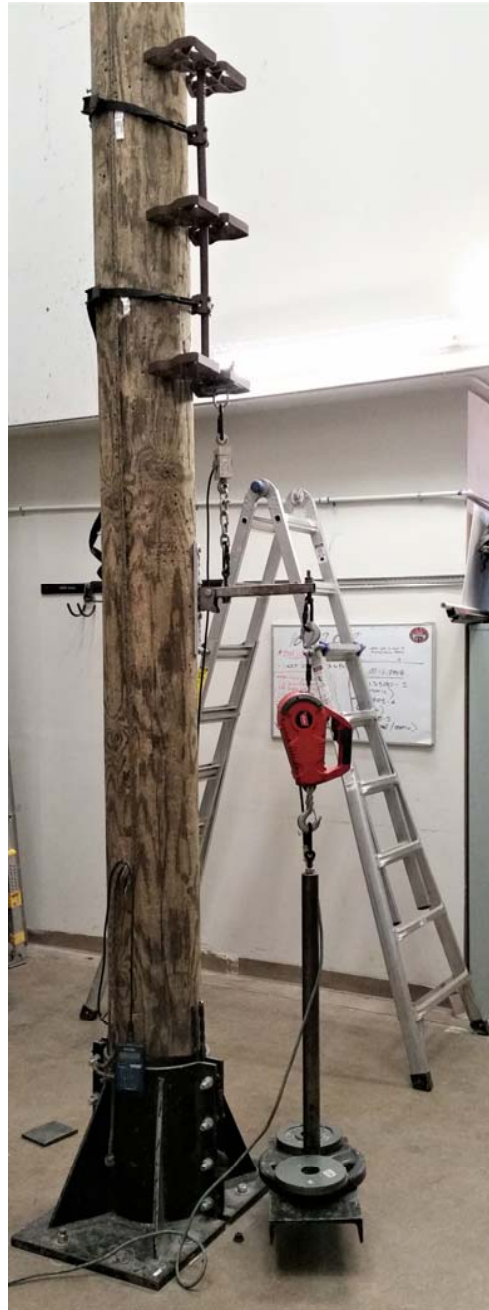
Photo 5 – Static Load Testing
