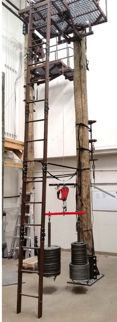
Photo 4 – Static Load Testing of Platform
