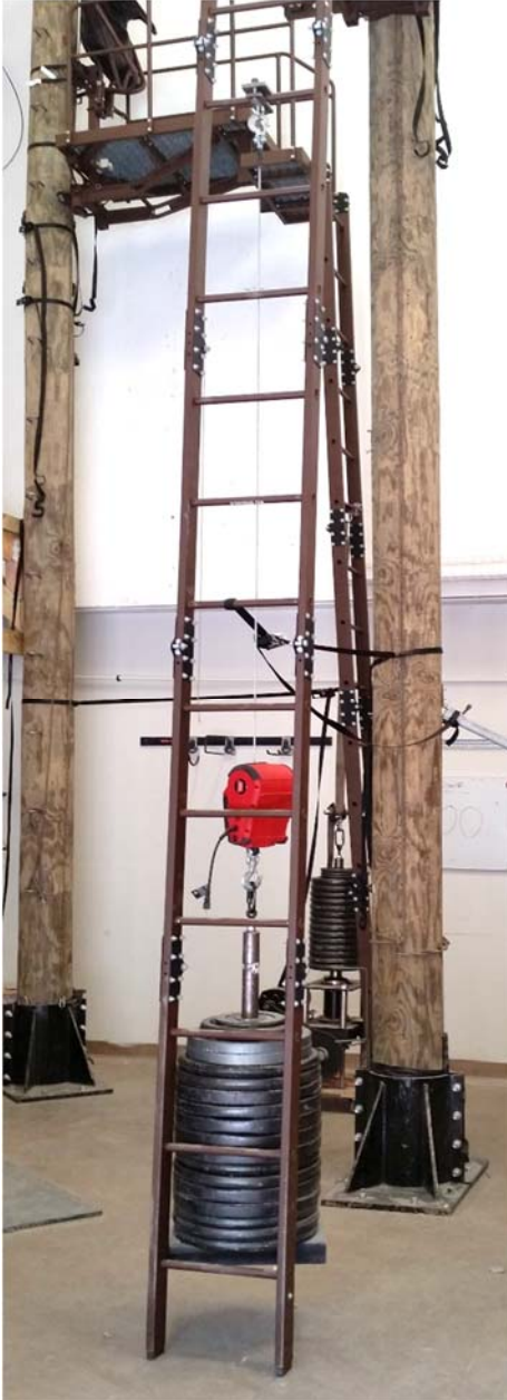
Photo 3 – Static Load of Ladder Step
