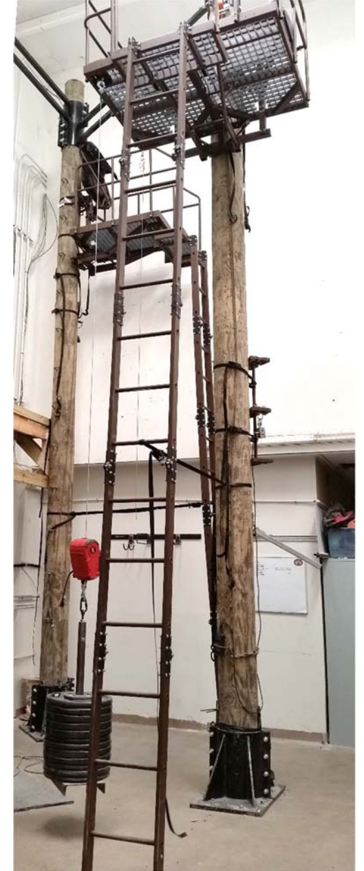
Photo 5 – Stability and Adherence Testing
