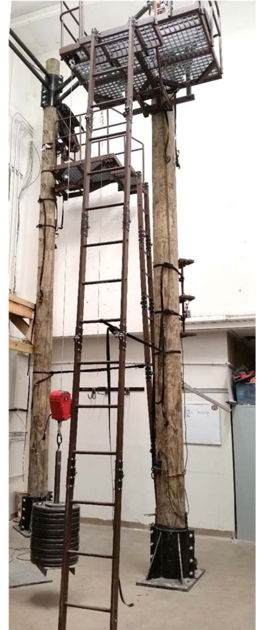
Photo 5 – Stability and Adherence Testing
