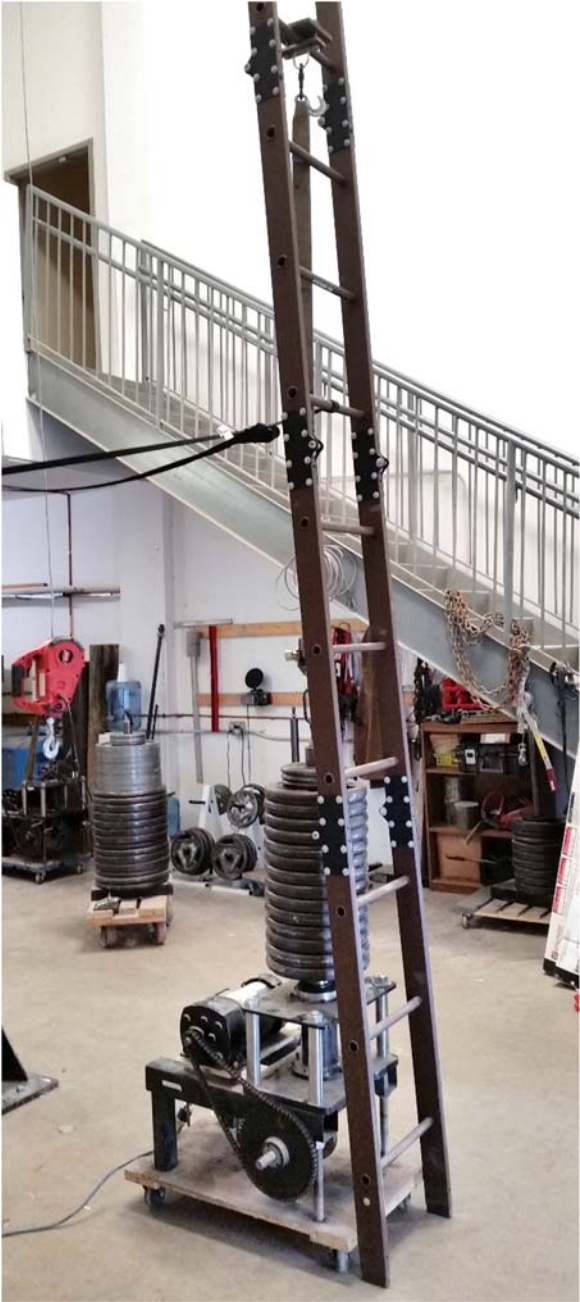
Photo 7 – Cyclic Load Testing
