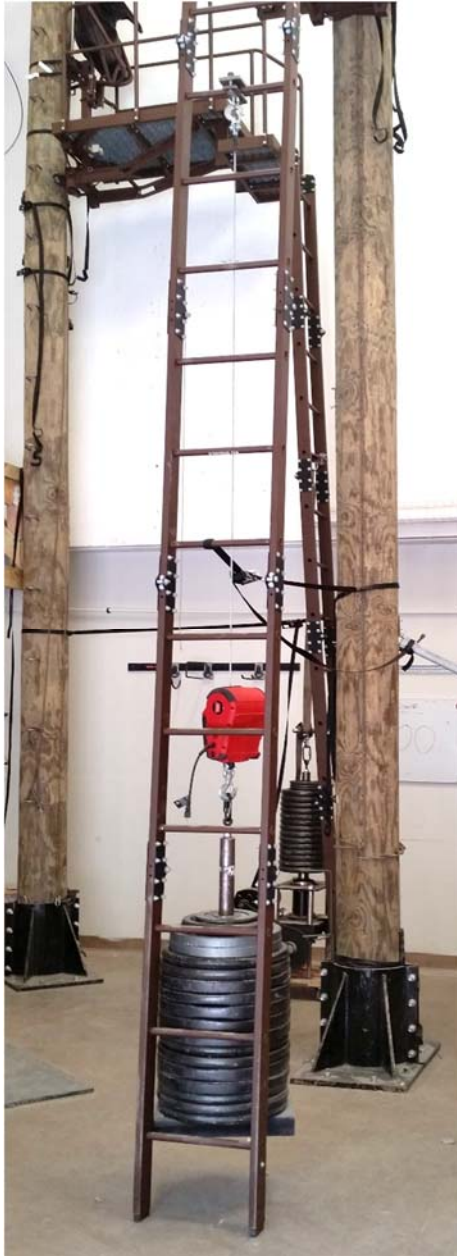
Photo 3 – Static Load of Ladder Step
