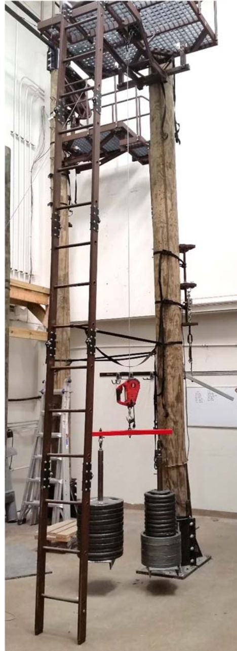
Photo 4 – Static Load Testing of Platform
