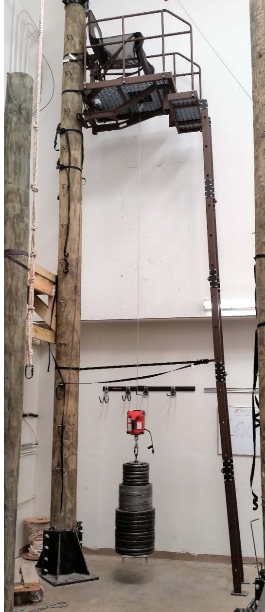
Photo 4 – Static Load Testing of Platform
