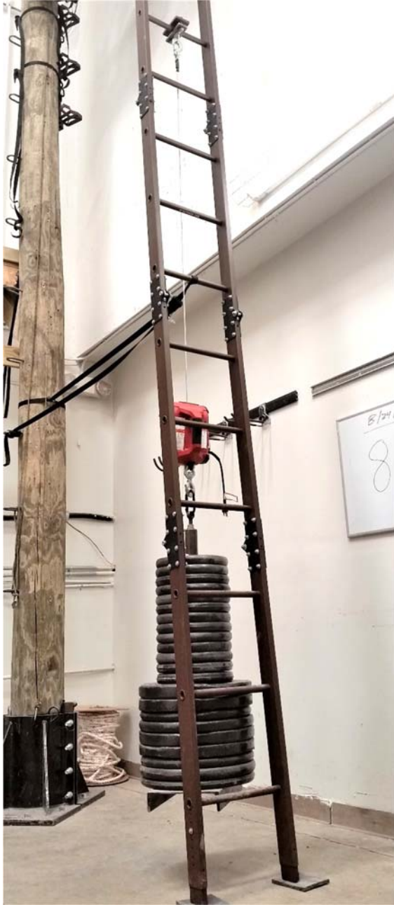
Photo 3 – Static Load of Ladder Step
