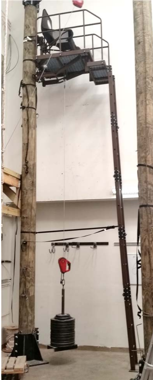
Photo 6 – Seat Load Testing
