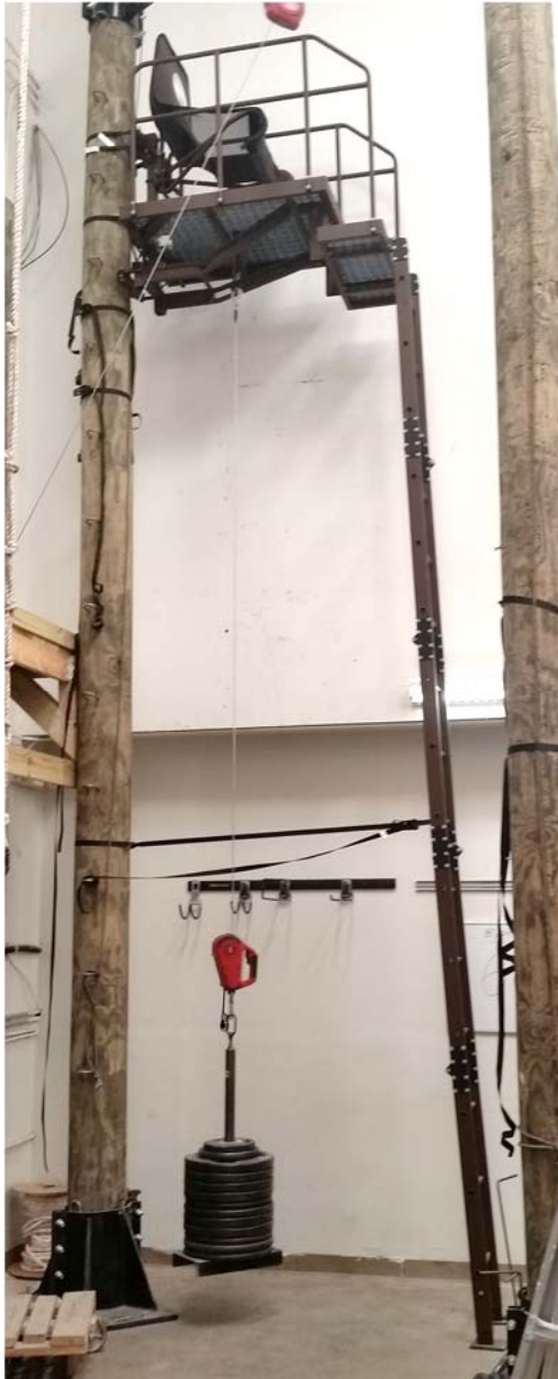
Photo 6 – Seat Load Testing
