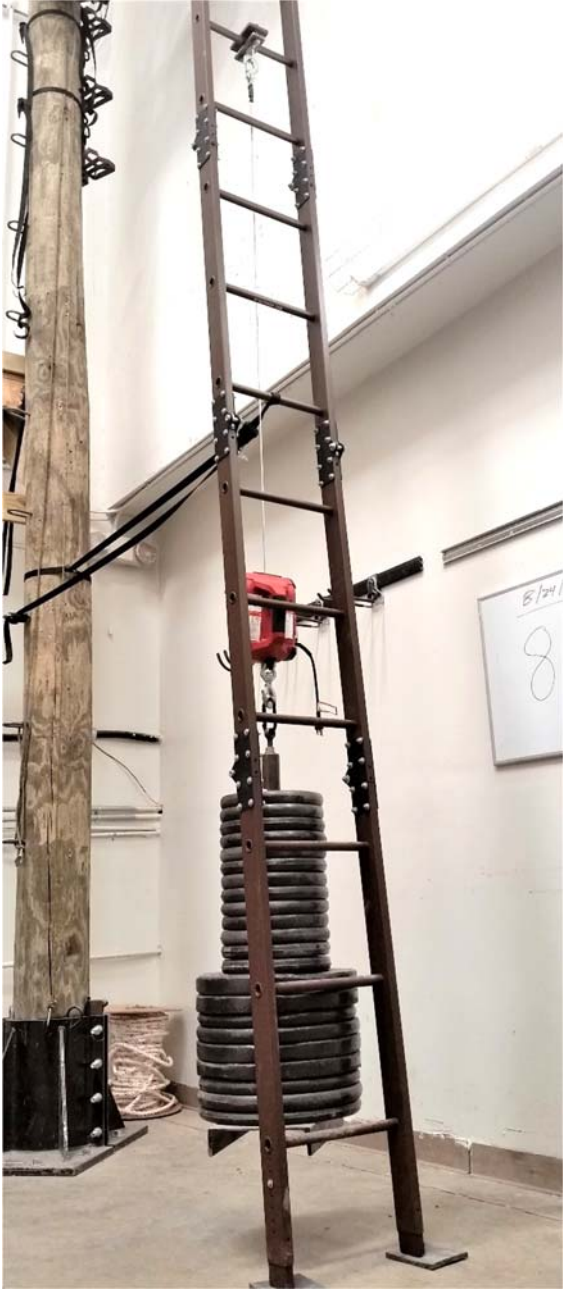
Photo 3 – Static Load of Ladder Step
