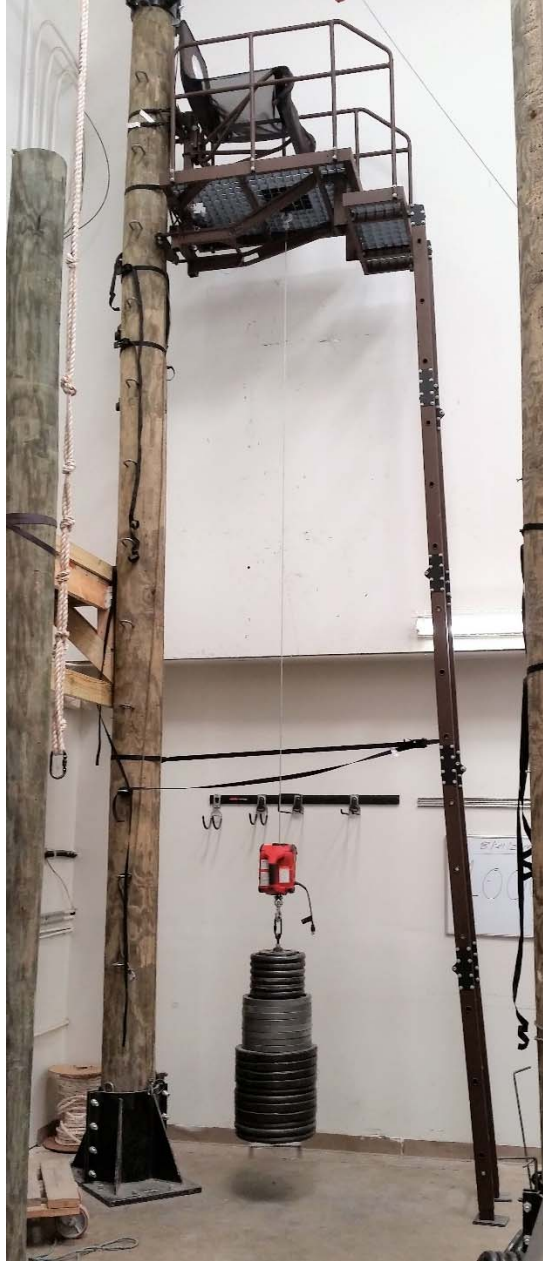
Photo 4 – Static Load Testing of Platform
