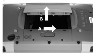
Remove the compartment door (B). Remove the battery.
