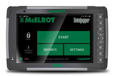
Capture the most important data from your fusion jobsite—no matter how long the workday. The DataLogger <sup>®</sup> 7 delivers increased battery life, automatic data backup, an updated Android operating system and more in a new, IP68-rated and MIL-STD-810 tested, rugged touchscreen tablet.
