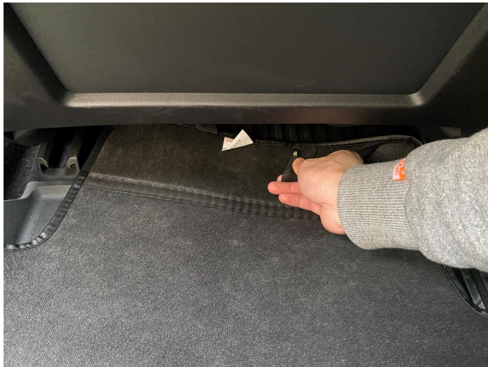
Step 3: Fix these two hooks under the seat. There are many places these hooks can be fixed on under the seat, look for the best spot using your hands. Adjust the alignment, installation done!
