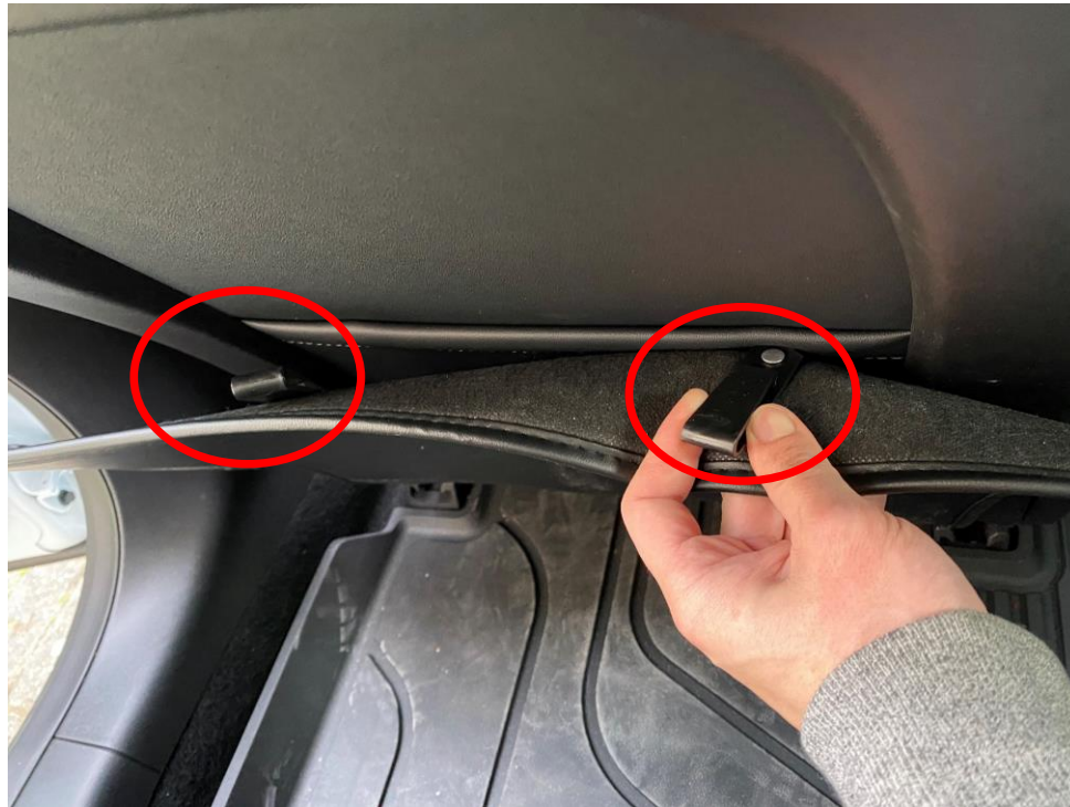
Step 1: Fix these two clips on the pocket edge
