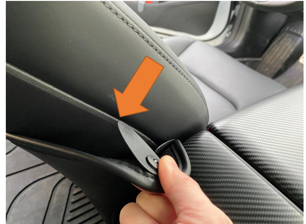
Step 2: Fix these two clips inside the gap between plastic part and leather part, do the same for the left side.
