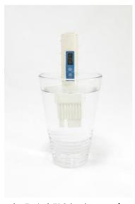
Many consumers ask about TDS meters - A TDS meter measures the electrical conductivity in the water, which can be correlated to the amount of total dissolved solids in the water. A TDS meter does not directly measure heavy contaminants such as lead or arsenic in the water. A TDS reading is not an indication as to whether a water filter is working properly to reduce these contaminants.
