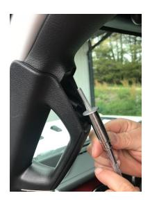
Step 3 Install the Mount that has the red dot into the handle and tighten the provided bolt with a 5mm Allen.
