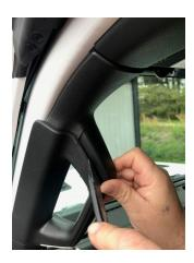
Step 2 Use an 10mm Socket to remove the bolt inside the handle.
