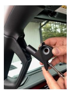
Step 4 Carefully re-install the 1" Ball mount and tighten with an 8 mm allen wrench. Do not exceed 180 in/lbs.
