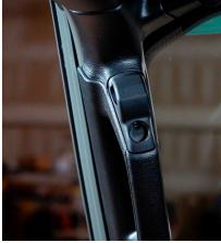
**Step 4** Carefully re-install the 1"or 20mm Ball OR Delete mount and tighten with an 8 mm allen wrench. Do not exceed 180 in/lbs
