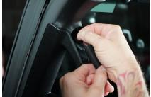
Step 2 Use an 10mm Socket to remove the bolt inside the handle.
