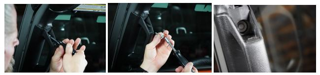
Step 3 Install the Mount into the handle and tighten the provided bolt with a 5mm Allen.
