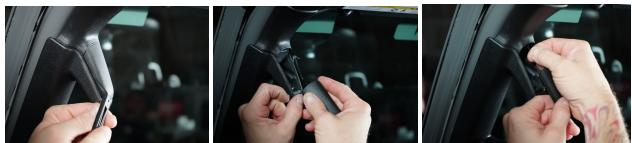
**Step 2** Use a 10mm Socket to remove the bolt inside the handle.
