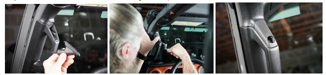
**Step 4** Carefully re-install the 1" or 20mm Ball mount and tighten with an 8 mm allen wrench. Do not exceed 180 in/lbs.
