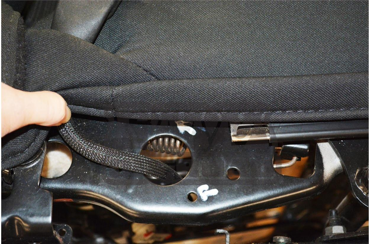
Step 4 Use the two 5/16" socket head cap screws and install the handle to the seat frame. Install the nuts and tighten.
