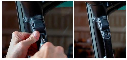
**Step 4** Carefully re-install the 1"or 20mm Ball OR Delete mount and tighten with an 8 mm allen wrench. Do not exceed 180 in/lbs
