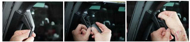
Step 2 Use an 10mm Socket to remove the bolt inside the handle.
