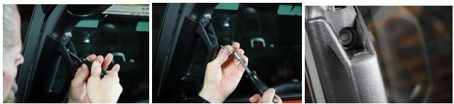
Step 3 Install the mirror base into the handle and tighten the provided bolt with a 5mm Allen.
