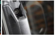
Step 3 Install the Mount into the handle and tighten the provided bolt with a 5mm Allen.
