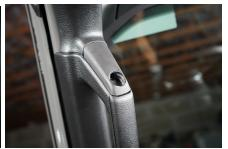
**Step 4** Carefully re-install the 1" or 20mm Ball mount and tighten with an 8 mm allen wrench. Do not exceed 180 in/lbs.
