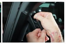
**Step 2** Use a 10mm Socket to remove the bolt inside the handle.
