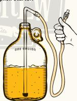
Place the clamped end of the tubing as low as possible and unclamp.
