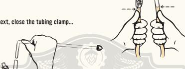
...and attach the non-clamped end to the racking cane; this will be your siphon starter.
