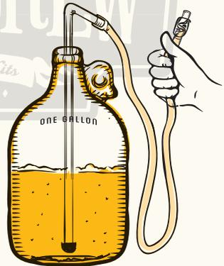
Place the clamped end of the tubing as low as possible and unclamp.
