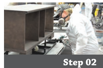
Step 02 Wood stain application
