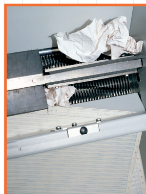
AUTOMATIC MECHANICAL FEEDING SYSTEM WITH REVOLVING FLAPS
