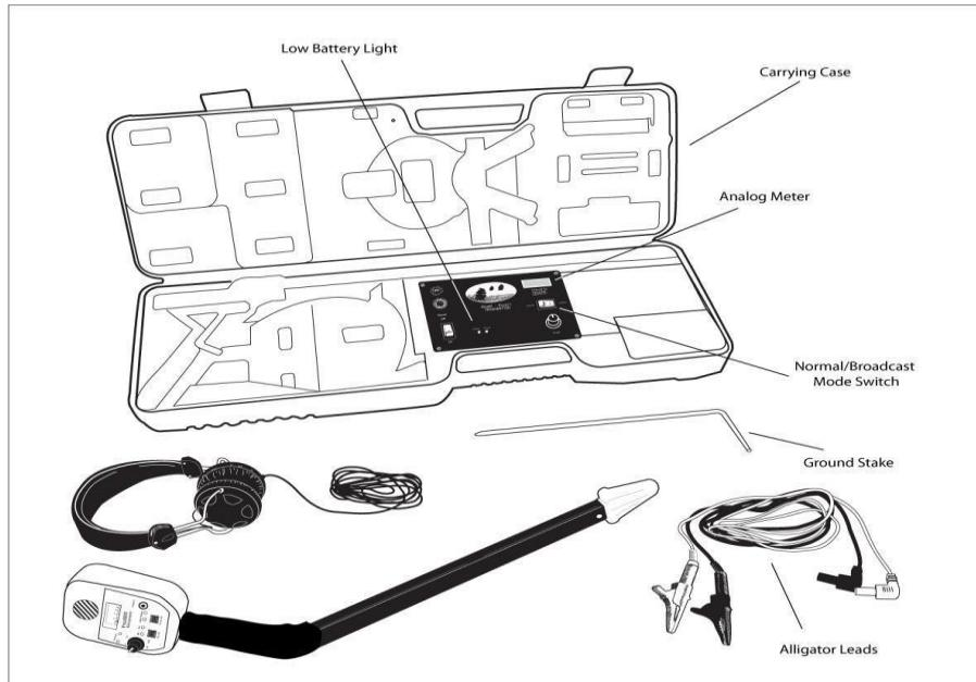
**Theory of Locating** - Cable Locators consist of a transmitter and a receiver. In the case of the Pro800D model, the transmitter is the long black box, and the wand is yellow and black. In operation, a transmitter places a specific frequency signal onto the metallic conductor you are trying to trace. This placing of an AC signal onto
