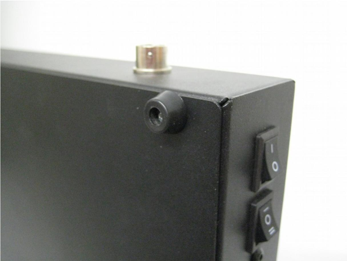
First batch with a detachable cable. Had rubber screw feet on the bottom. (Earliest versions had slightly different rubber screw feet) Important to note that Gen2 Smash Boxes use a different driver than Alpha, Gen1 and Gen3. Install the Teensy drivers for this board. Most computers already have this driver installed.
