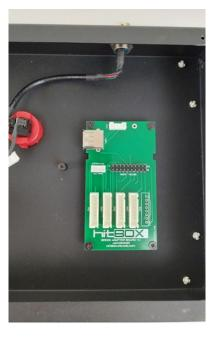
The adapter fits over the mounting posts using the same bolts that you took out of the original breakout.
