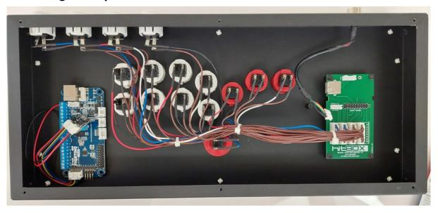
In the above example, the PS4 Audio+ Fighting Board has a layer of gaffing tape on the underside of the board and is fastened to the case with double-sided mounting tape. The Brook UP5 board is also insulated with gaffing tape and is fastened directly to the Audio+ board using Loctite Mounting Putty.
