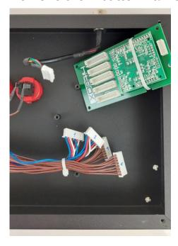
The button wire harnesses are usually (but not always) numbered. The Hit Box breakouts connectors have the designation CN1, CN2, CN3, CN4 and or CN5 above each connector. Make sure you know which harness attaches to which connector because the adapter kit retains this connection scheme.
