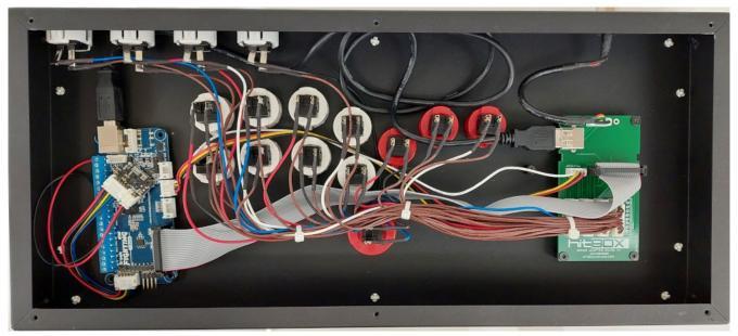
The included USB cable will connect your alternate PCB to the Hit Box case USB port. Our existing detachable cable can then be used on any system that connects through USB.
