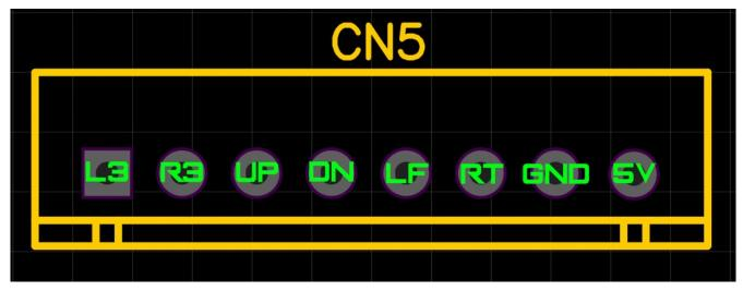
The unpopulated connector breaks out L3, R3, the 4 dpad directions, along with a ground and 5v line. These ports can be tapped for any number of mods (LEDs, optical switch boards, adding extra directional buttons, adding dedicated L3/R3 buttons). Again, all mods are performed at your own risk.
