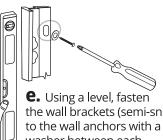
the wall brackets (semi-snug) washer between each screw and wall bracket.
