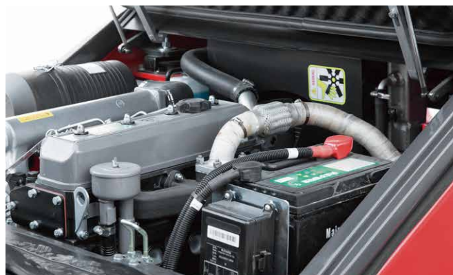
Fully opening up of bonnet reveals the convenient access to mechanical components for simplified maintenance.
