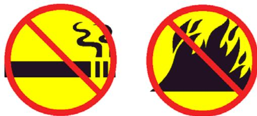
Keep sparks, flames and lighted tobacco away from batteries. Batteries emit explosive gas.
