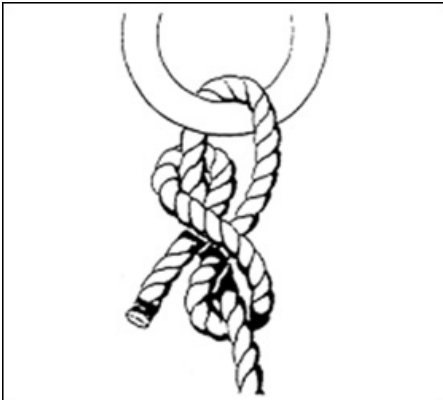
Buntline hitch: Secure method of securing a rope to a ring or tube.
