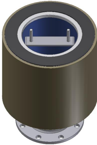
Figure C.3.1: Element sitting in housing base.
