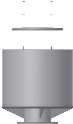
Figure C.3.1: Removal of hex nut, washer, and top plate.
